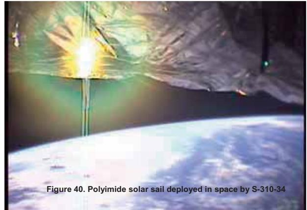
Figure 40. Polyimide solar sail deployed in space by S-310-34
