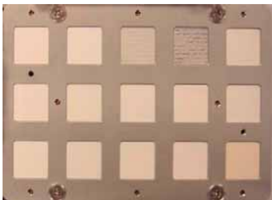
Fig. 33 Pre-flight photograph of the MISSE 6B New Thermal Control Paints Experiment.
