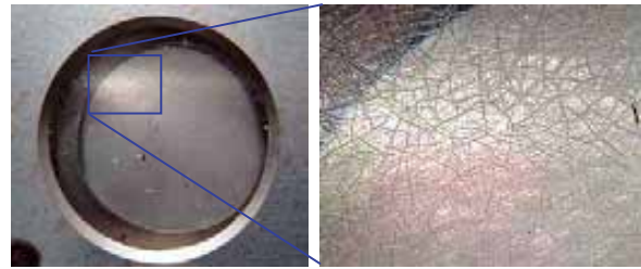
Fig. 8 Post-flight photograph of MISSE 2 DC 93-500 sample 2-E5-1 showing the crazed surface.
