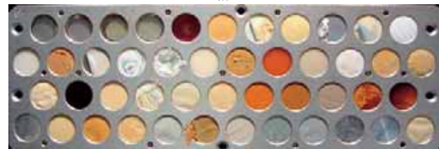
Fig. 7 MISSE 2 PEACE Polymers experiment (Sample Tray E5), a). Prior to flight, and b). After space flight.
