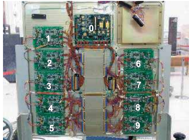
Fig. 20 Photograph of the DAC (1-9) boards and main microprocessor board (0) that perform the FTSCE electrical measurements. The metal box in the upper right is the power control unit (PCU). The metal boxes in the center route wires from the solar cells mounted on the opposite side and serve to maintain a Faraday cage around the measurement electronics.[18]
