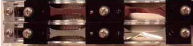
Fig. 24 Two sets of tensile test samples in fixtures on MISSE 6 Polymer Film Tensile Experiment. For each set, the left hand sample is installed in a spring-loaded fixture to apply stress and the right hand sample is installed with no tensile stress applied.
