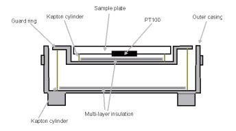
Figure 6 Micro-calorimeter schematic
