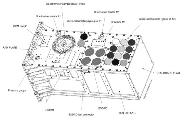
figure 1 : Schematics of MEDET experiment
