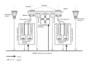
Figure 2 : Spectrometer experiment interface schematic
