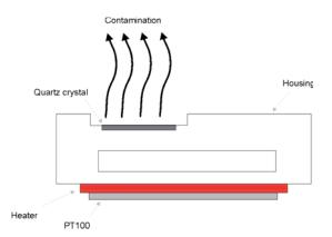
Figure 4 : QCM sensor in regenerate mode
