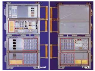
Figure 3 Photographs of SM/MPAC&SEED (570 (W)×900 (H)×156 (D) [mm])
