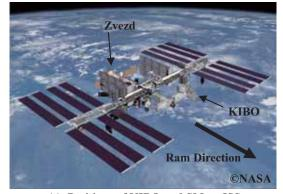
(c) Positions of KIBO and SM on ISS Figure 1 External views of KIBO and Zvezda
