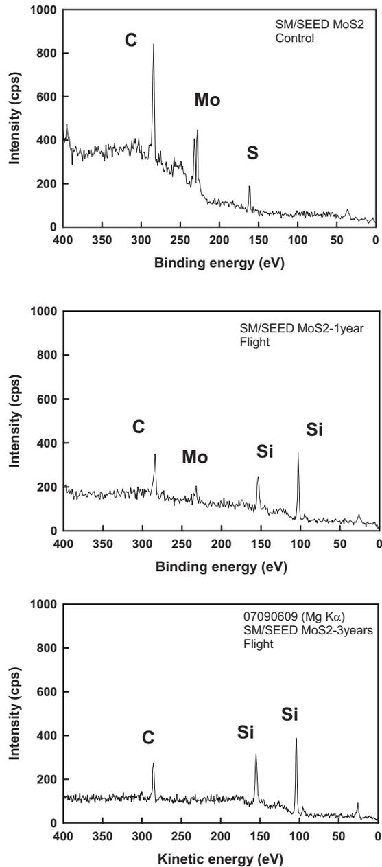
Fig.1 X-ray photoelectron spectra of control, 1-year and 3-year-exposed samples of MoS<sub>2</sub> aboard SM/MPAC&SEED.
