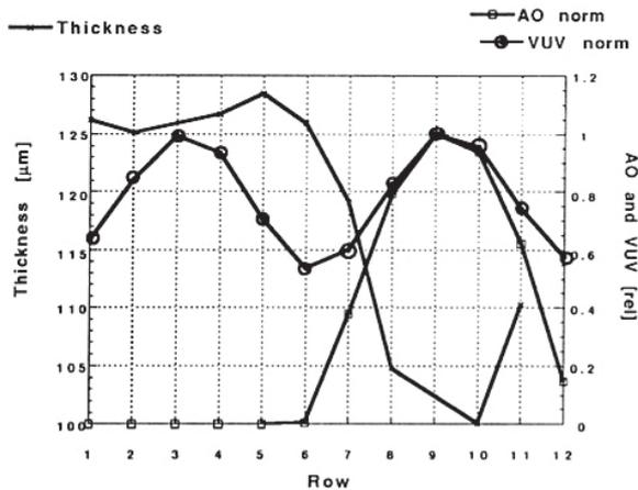
Fig.3 LDEF results regarding FEP Teflon degradation [8].
