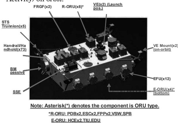
Fig.2 JEM-EF Subsystems
