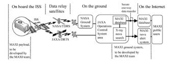
Fig. 1. The MAXI system. We have two downlink paths for the MAXI data. The MAXI team is responsible for the MAXI payload and its ground system. The MAXI mission, including the rapid distribution of observational results. The MAXI data will be transmitted to the Internet through a secure one-way path. Teaming up with public users is also an important task of the MAXI team for follow-up observations.
