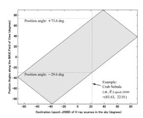
Fig. 5. The coverage of the field of view for a source with given declination angle. For example, Crab nebulae, a useful calibration source in X-ray astronomy, moves across the FOV at the position angles between -29.6 degrees and +73.6 degrees.
