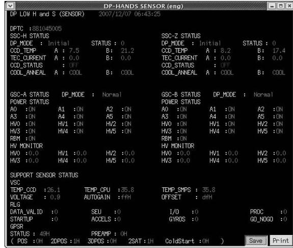
Fig. 4. The sample of QL display (Engineering Value)
