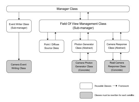
Fig. 2. The schematic structure of the MAXI simulator.
