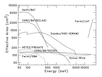
Fig. 2. On-axis effective area of the Suzaku WAM in comparison with previous and current GRB detectors. The Suzaku WAM has a very large effective area ∼400 cm² in the MeV range.
