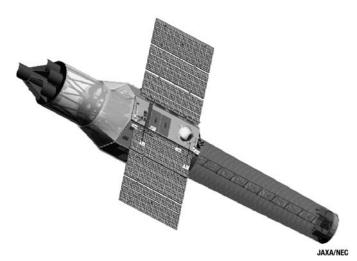
Fig. 1. Artist's drawing of the ASTRO-H satellite. The focal length of the Hard X-ray Telescope (HXT) is 12m, whereas the Soft X-ray Spectrometer (SXS) and Soft X-ray Imager (SXI) will have a focal length of 6 meters.
