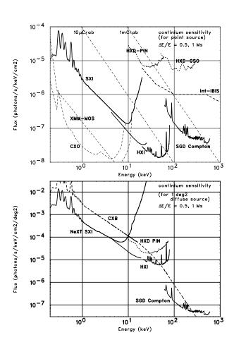
Fig. 4. Detection limits of the SXT-I/SXI and HXT/HXI for (a) point sources and (b) for sources with of  $1\!\times\!1~{\rm deg}^2$  extension (bottom) as functions of X-ray energy, where the spectral binning with  $\Delta E/E=0.5$  and 1000 ksec exposure are assumed. Detection limits for the XMM-Newton, Chandra, Suzaku and Integral observatories are shown for comparison for the sensitivity for point sources.
