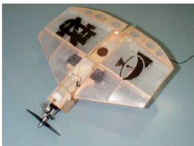
Fig. 1 Example of MAV (body length=24.8cm, weight=105g, developed at Notre Dame University, USA)
