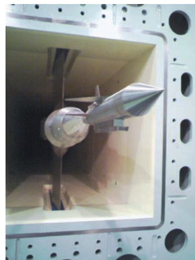
Fig. 3 : A 9/100-scale wind-tunnel model of BOV 3 attached to the sting in the 2 × 2 m supersonic wind tunnel at ARD/JAXA.
