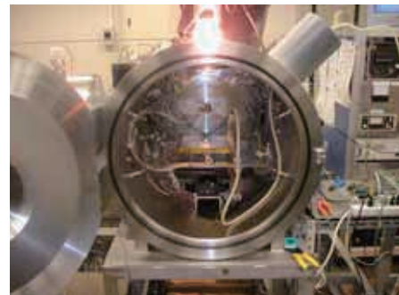
Figure-6 MD cell array coupon in the test chamber
