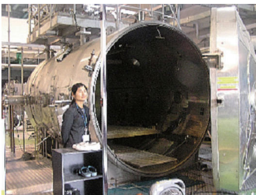
Fig. 1. A photograph of the space-plasma chamber in ISAS/JAXA.
