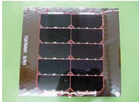
Figure-5 Coupon panel for ESD Test
