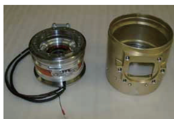
New joint mechanism & torque sensor
