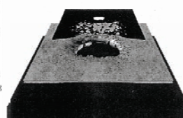
Fig. 9. Element plot of the simulation results at 75 microseconds after impact (front view).
