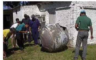
Titanium casing of the STAR-48B solid rocket motor found in northeastern Argentina.
