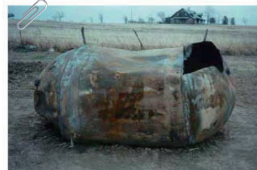
Delta II second stage propellant tank found in Texas, 1996
