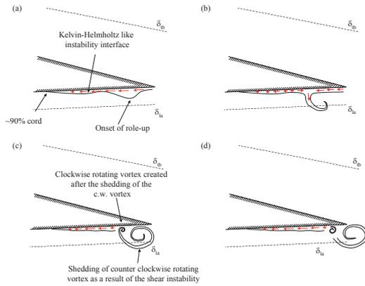
**Figure 1: Schematic of the tonal noise generation process**
