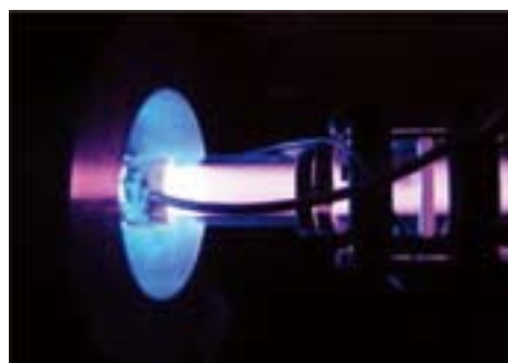
Fig.10 Compact helicon plasma in blue-mode in a 2.5cm i.d glass tube.
