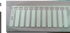
External stress type whisker test sample (put into SEM, directly observable)
