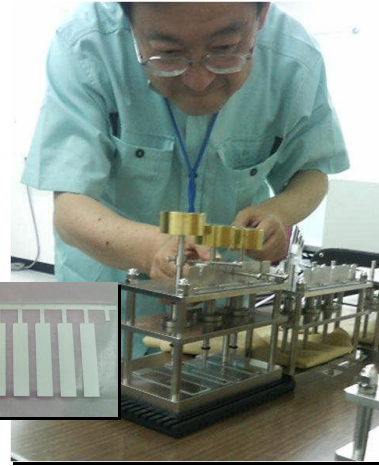
External stress type whisker test sample (put into SEM, directly observable)
