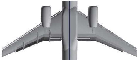
Fig.2 JAXA High-Lift configuration model (left: with clasps right: without clasps)
