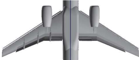
Fig.2 JAXA High-Lift configuration model (left: with clasps right: without clasps)
