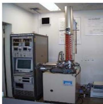
Outgas measurement test apparatus
