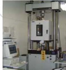
Tensile, Compress and Fatigue Testing Machine
