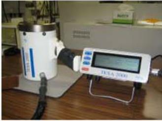
Total Emittance / Solar Absorptance Portable Reflectometer
