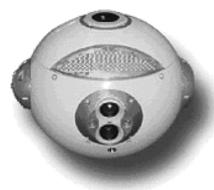
Miniature Autonomous Extravehicular Robotic Camera (Mini AERCam, NASA JSC)
