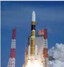
**H-IIA Launch Vehicle** H-IIA launch vehicle is the Japan's primary large rocket equipped with high performance engines that use liquid oxygen and hydrogen as propellants.
