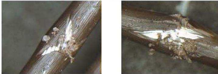
Covering cracked after heating with soldering iron
