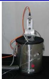
Vibration Test; MTP Connector
