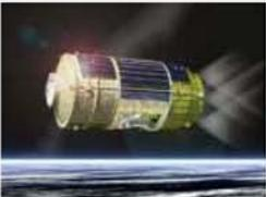
**HTV** HTV(H-II Transfer Vehicle)is a re-supply vehicle for the ISS. HTV is an unmanned vehicle designed to be attached on top of the augmented H-IIA launch vehicle, delivers a maximum of 4 tons of foods, clothes and various experiment equipment to the ISS and brings back used experiment equipment and clothes to the atmosphere. HTV will be burnt during the re-entry.
