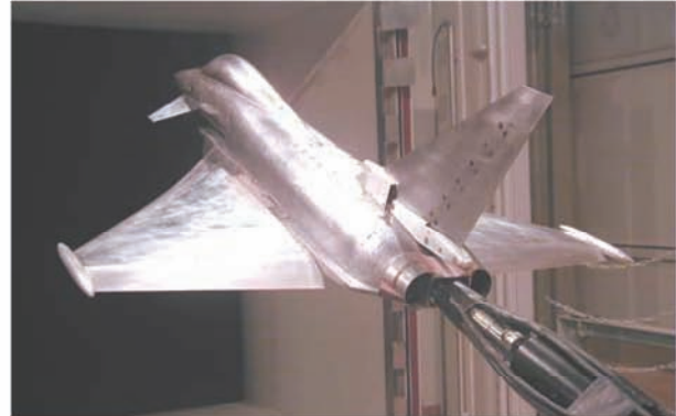
Figure 12: Wind tunnel test of a fighter aircraft model with simulated adaptive trailing edges.
