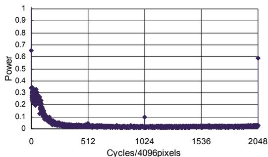
Fig. 2.1.3-4 Power spectrum of PRISM nadir image (CCD #4).
