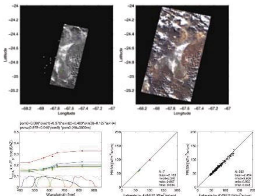
Fig. 2.1.3-7 Cross calibration of PRISM (upper left) with AVNIR-2 (upper right) over Arizaro, Argentina, and comparison of radiances between PRISM and AVNIR-2 (lower center and right).
