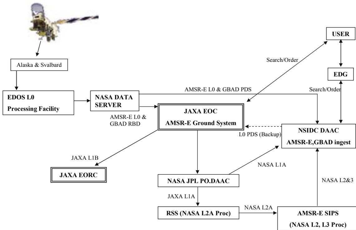
Fig. 3.2.2-1 Schematic view of AMSR-E data flow.
