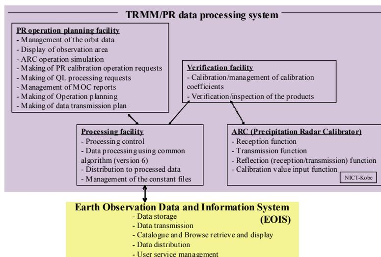
Fig. 3.2.1-2 Overall structure of TRMM/PR data processing system.
