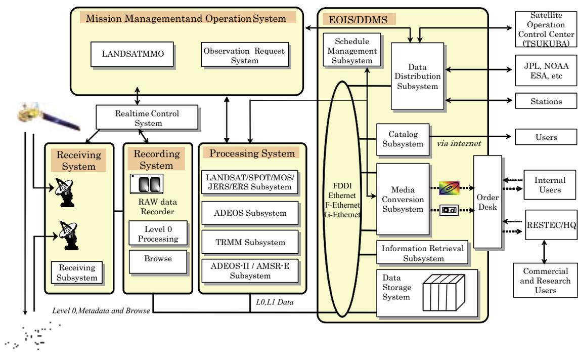
Figure 3.1.2-1 Schematic of the EOC system.
