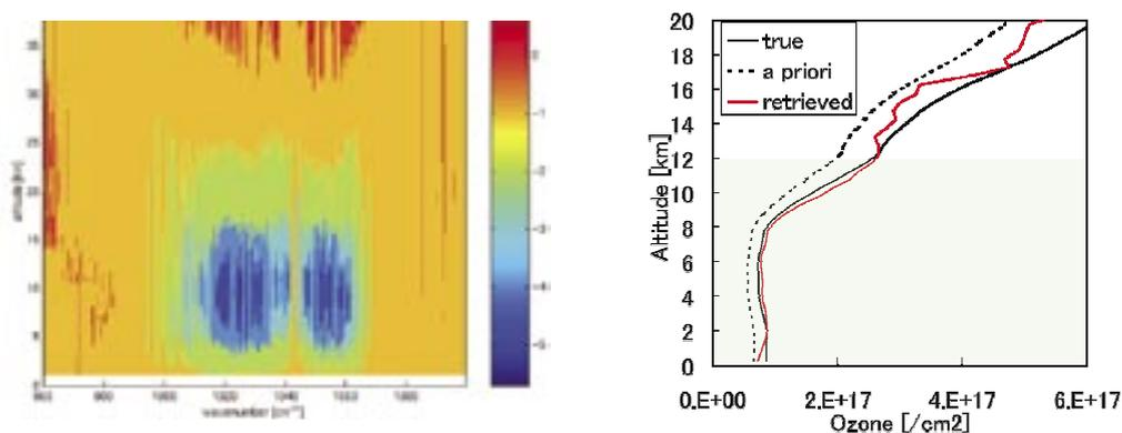
Fig. 2.1.4-4 O<sub>3</sub> retrieval test with TANSO-FTS specification: O<sub>3</sub> weighting function (left), and the result of the O<sub>3</sub> retrieved profile (right).
