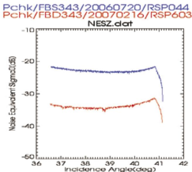
Fig. 2.1.3-19 Noise equivalent sigma-naught vs. incidence angle. Blue: Greenland by FBSHH. Red: Hawaii by FBD-HV.
