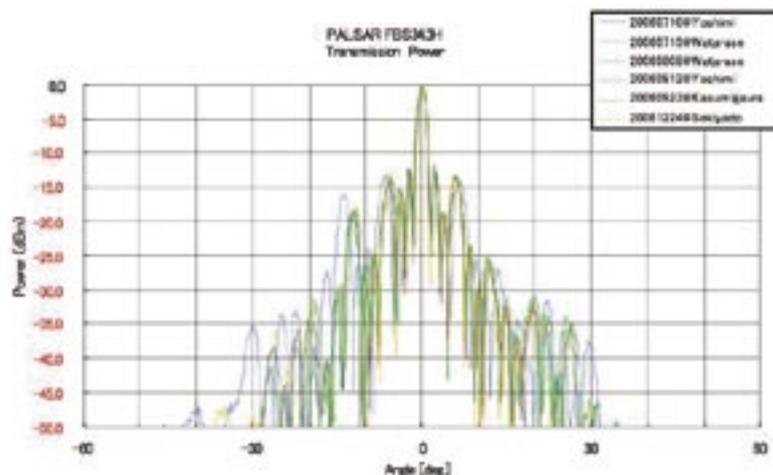
Fig. 2.1.3-13 Measured azimuth antenna pattern (in HH pol). Red curve and Blue curve are real measurement and the ground measurement.
