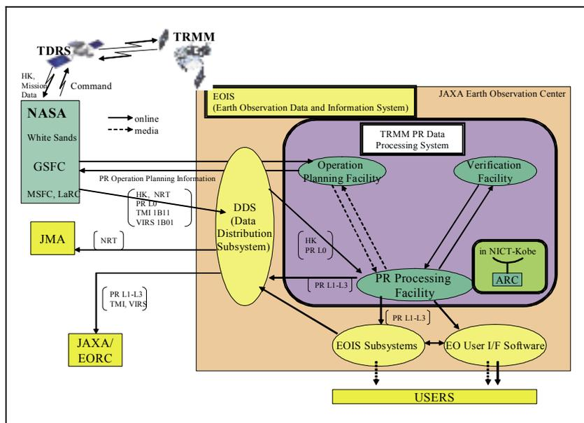
Fig. 3.2.1-1 TRMM Ground System Configuration.
