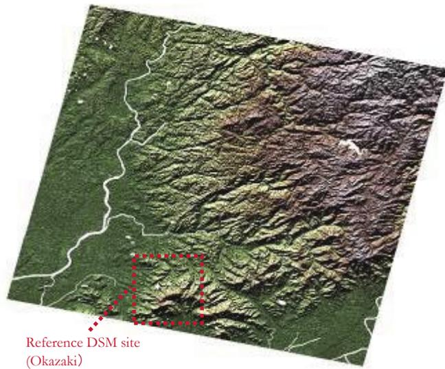
Fig. 2.1.3-10 Color shaded PRISM-DSM of scene 2 (35km x 35km).
