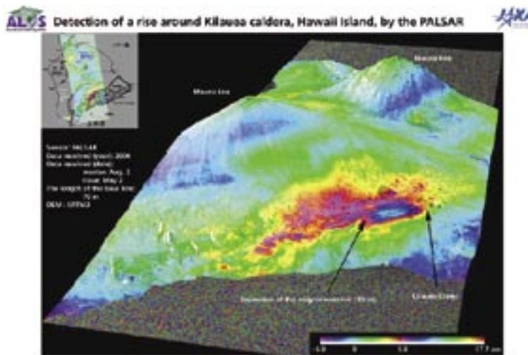
Fig. 2.1.3-31 Crustal deformation at Kilauea caldera, Hawaii, between May 2 and Aug 2, 2006 detected using PALSAR.
