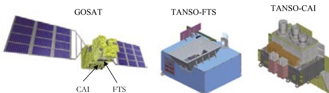
Fig. 2.1.4-1 GOSAT satellite and TANSO instruments: GOSAT satellite (left), Fourier Transform Spectrometer (center), and Cloud and Aerosol Imager (right).
