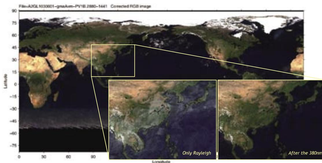
Fig. 2.1.2-16 Performance of the atmospheric correction scheme with and without using 380nm channel (GLI channel 1) reflectance.
