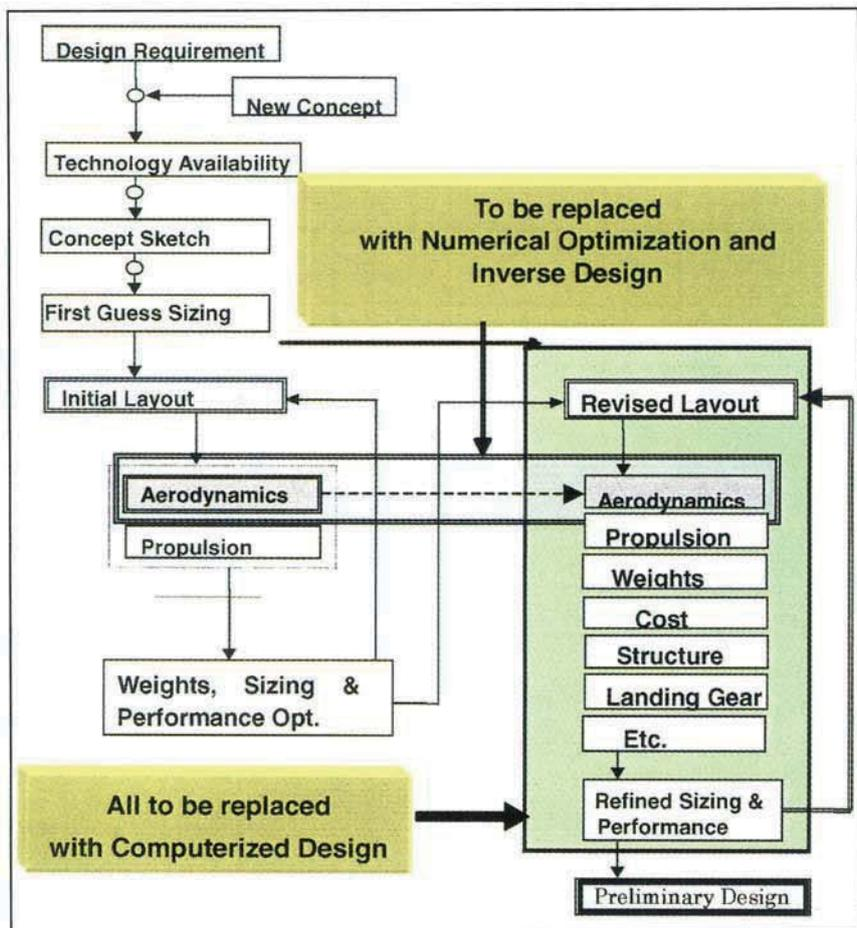
Figure 3 Conceptual design process and its modernization
