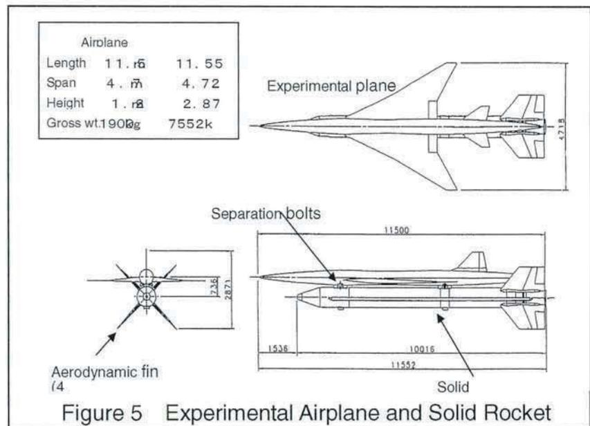
Figure 5 Experimental Airplane and Solid Rocket
