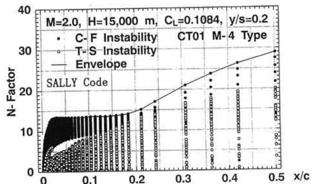
Figure 1. N characteristics estimated by SALLY code at 20% semi-spanwise station of the designed NLF wing
