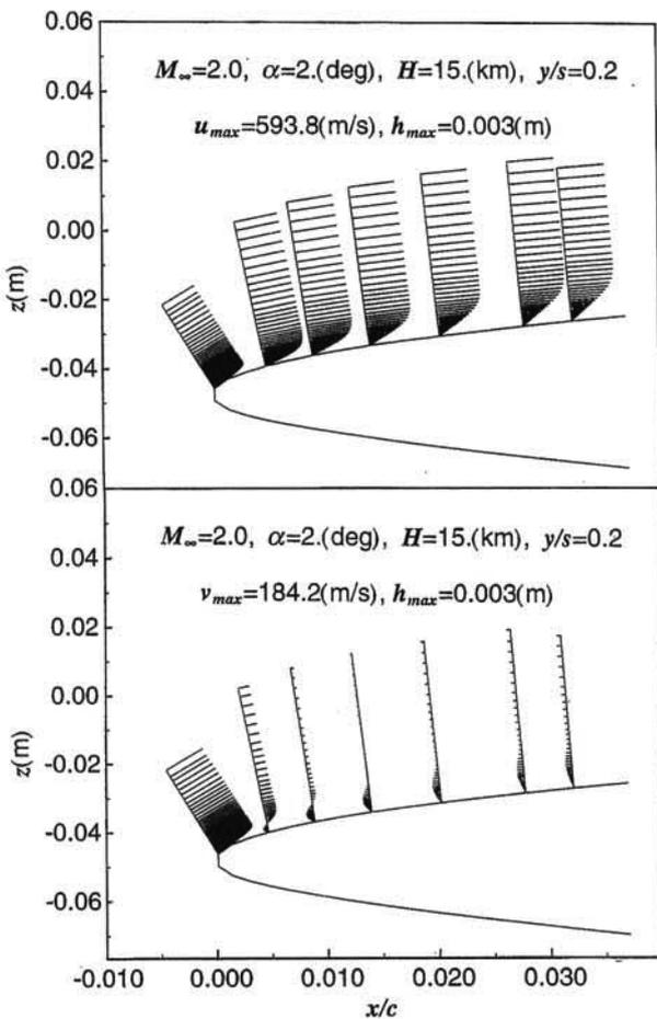
Figure 11. Laminar profiles estimated by N-S calculation
