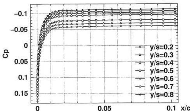
Figure 3. Target Cp distributions for supersonic NLF wing design at M=2.0, CL=0.1
