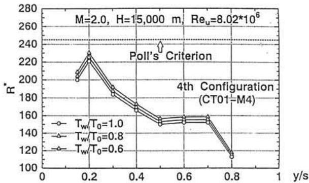
Figure 14. Result of consideration on attachment-line contamination
