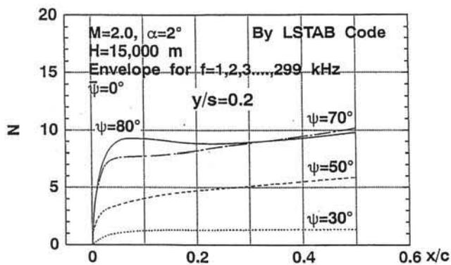
Figure 9. N characteristics estimated by LSTAB code at 20% semi-spanwise station of the designed NLF wing
