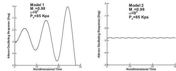
**Fig. 4 Dynamic responses of aileron oscillation for Model 1 and 2 at  $M_\infty = 0.98, \alpha = 0^\circ, P_0 = 85Kpa$**
