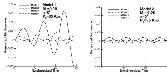
**Fig. 3 Dynamic responses of generalized displacement for Model 1 and 2 at  $M_\infty = 0.98, \alpha = 0^\circ, P_0 = 85Kpa$**
