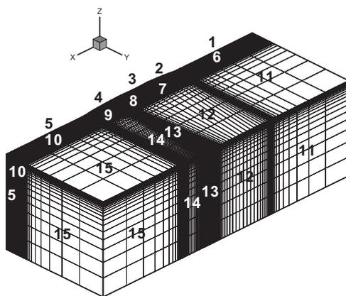
**Fig. 1 Multiblock grid with 30 blocks for SST**
