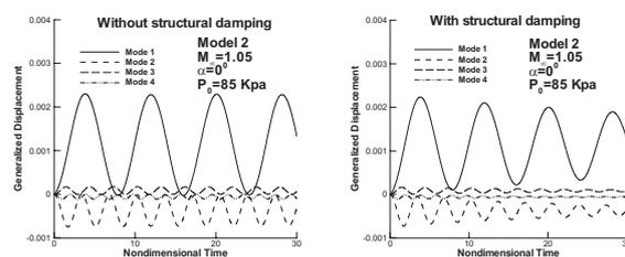
**Fig. 5 Dynamic responses with and without structural damping for Model 2 at  $M_\infty = 1.05, \alpha = 0^\circ, P_0 = 85Kpa$**
