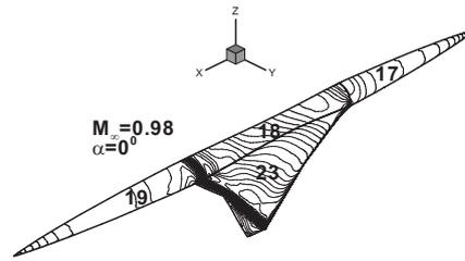
**Fig. 2 Pressure contour of steady flow for SST**
