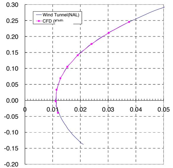
Fig.4 Comparison of lift vs. drag polar curve.
