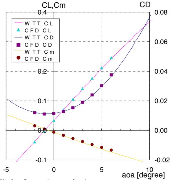
Fig.3 Comparison of three component force coefficients between CFD and WTT.
