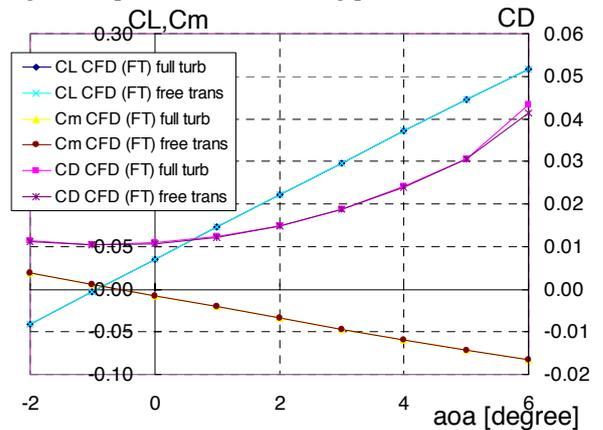
Fig.5 Calculated three component force coefficients for FT condition.
