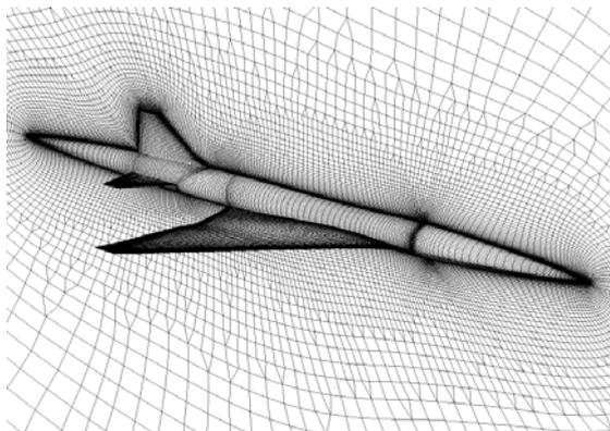
Fig.2 Surface and symmetry plane grid of NEXST-1
