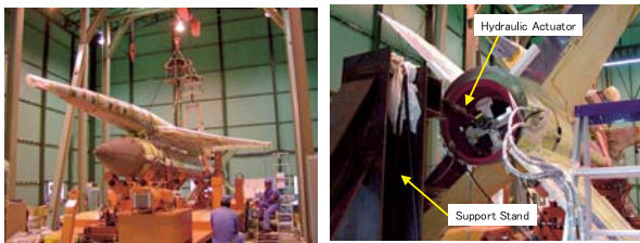
Fig. 12 Vibration test for the launch configuration
