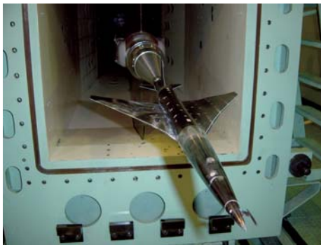
Fig.4 8.5% scaled model in wind tunnel test
