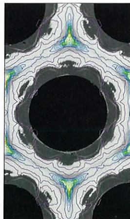
Simulated erosion contours overlaid on measured erosion pattern
