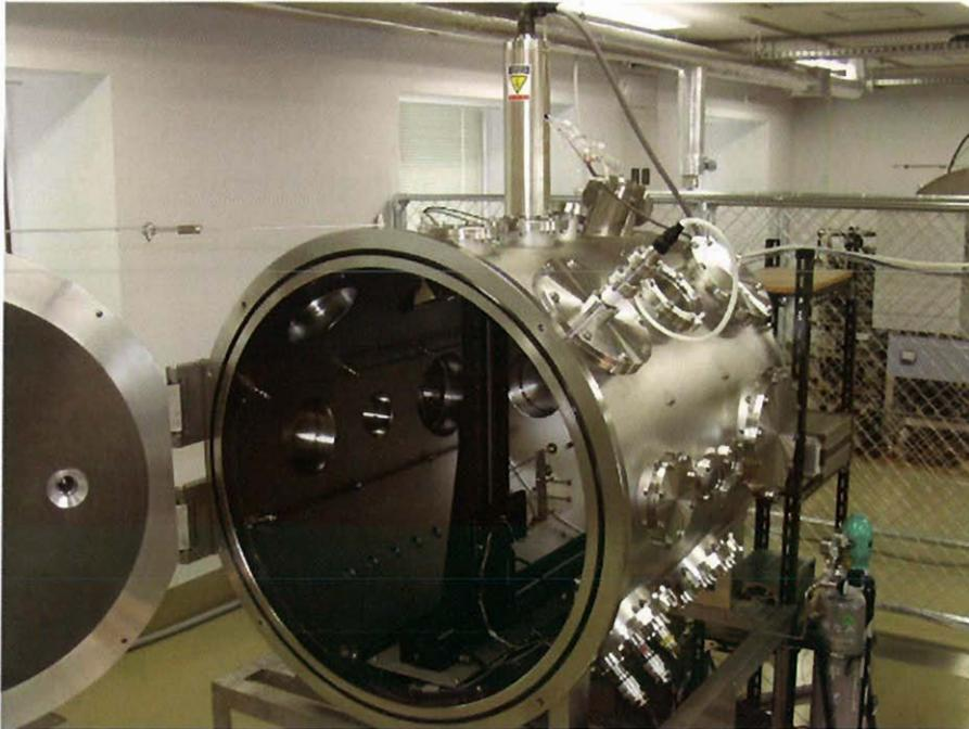
Chamber to simulate Polar Earth Orbit Environment 36
