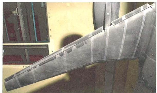
Fig.5 China-clay visualization (60m/s, AoA=10deg)
