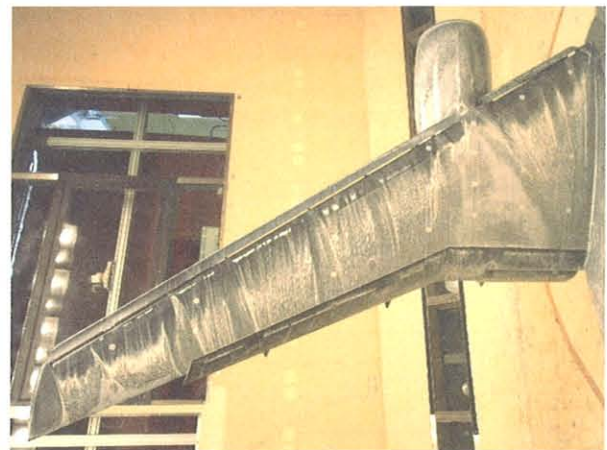
(a) Oil-flow visualization (60m/s, AoA=15deg)
