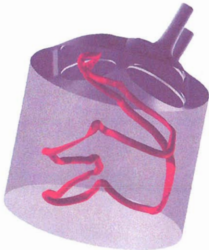
Fig. 4. Vortex loops, generated during the intake stroke in a four-valves engine near the lower dead center, after interaction with each other; computed with the solution described in [9]
