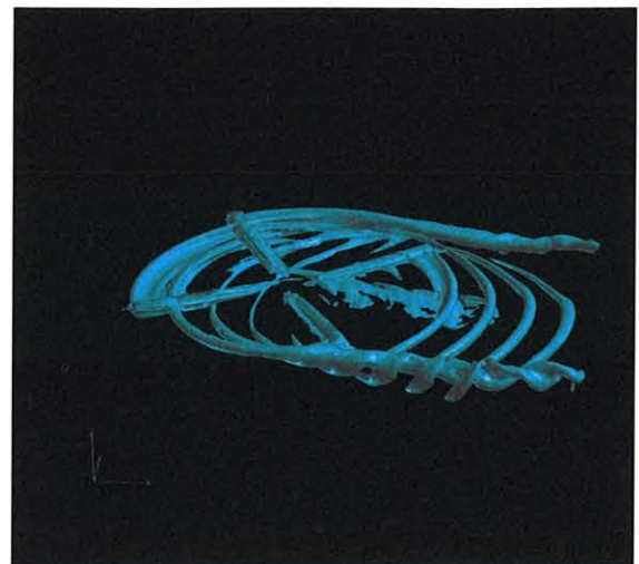
Fig.2 Iso-surface of vorticity magnitude
