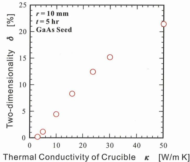
Fig. 9 Dependency of Two-dimensionality on thermal conductivity of crucible
