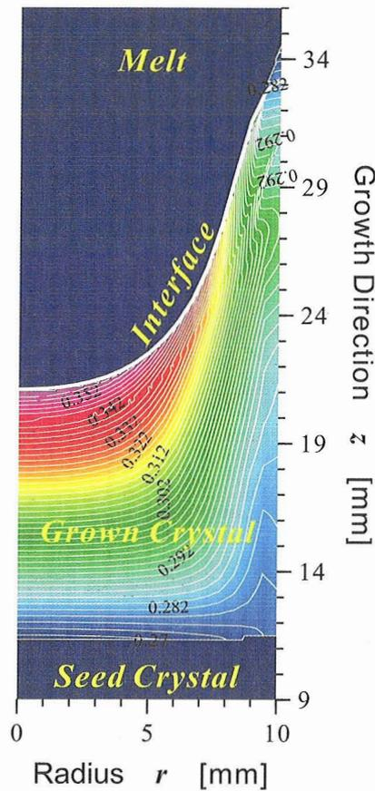
Fig. 4 Concentration distribution in grown crystal under no gravity condition
