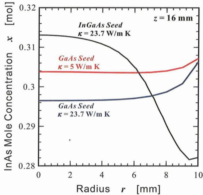
Fig. 8 Radial concentration profiles in grown crystals
