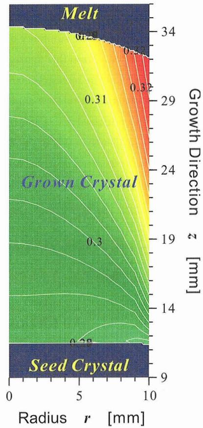
Fig. 6 Concentration distribution in grown crystal under no gravity condition
