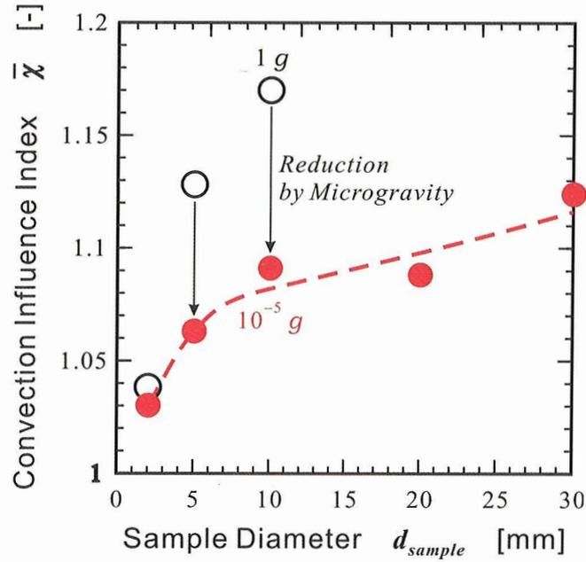
Fig. 1  $\bar{\chi}$  dependency on sample diameter
