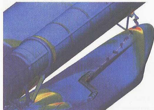
Time-dependent, moving-body simulation of foam debris impacting orbiter wing leading-edge.
