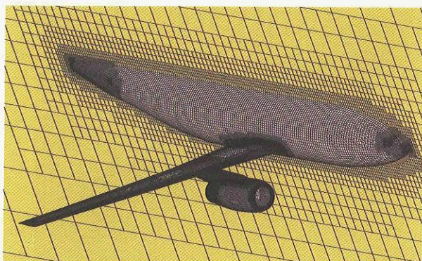
Figure 18. Overall view of the hexahedra grid around DLR F6.
