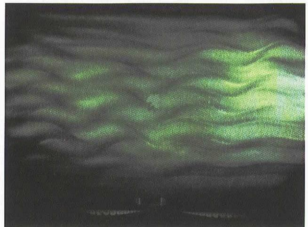
Figure 3. Roll-cells with large-scale wavy pattern. Vertical dimension of roll cells is approximately 2h. Re=100, Ro=0.05.
