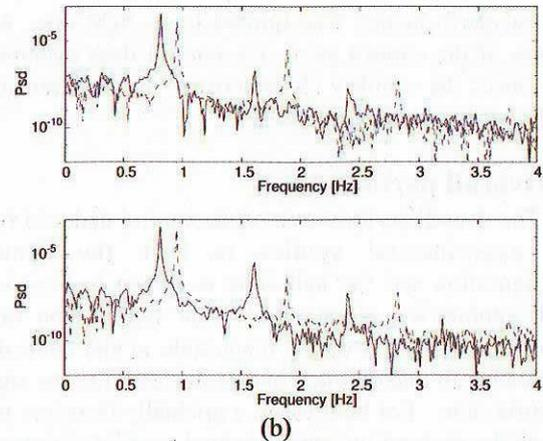
Fig. 5. The power spectrum density for the nondimensional temperature signal for both sensors. Dashed lines: without control. Solid lines: subjected to the linear control with,  $\text{Gain}=-0.155$  W (a) and  $\text{Gain}=-0.503$  W (b). Heater length,  $L_h = 1.5$  mm.  $\epsilon=0.24$ .
