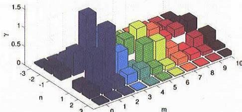
Fig. 4 Broadening of the spectra of the oscillation subjected to the linear control. The spatio-temporal decomposition of the oscillation in the numerical simulation.  $\gamma$  is the suppression ratio.  $\epsilon = 0.07$ .
