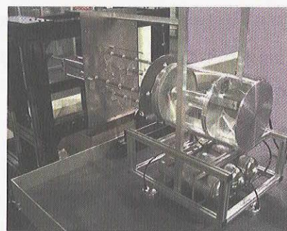
Fig.7 Prototype of tether reel mechanism
