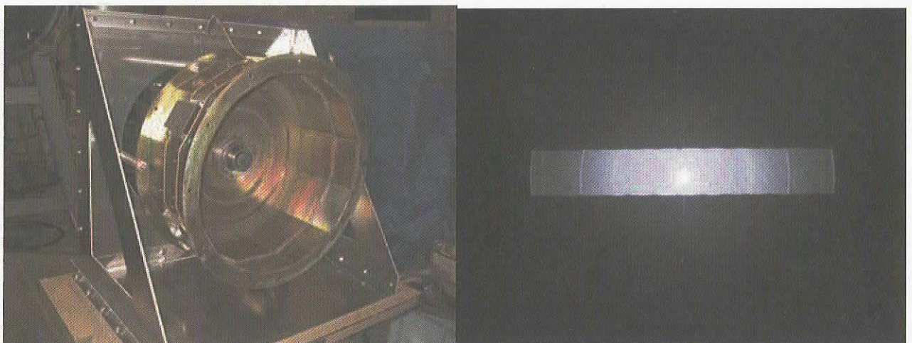
Fig. 3 Main Hollow Cathode in Discharge Chamber for Standalone Testing (Left) and Discharge Luminescence through Masked Fake Grid (Right)
