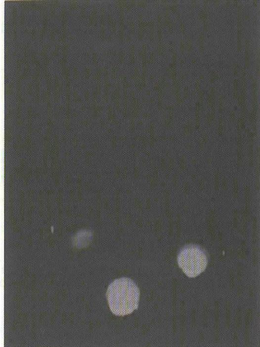
Fig.10 Plasma ignition during 45hour for thermal equilibrium on the thermal vacuum test.
