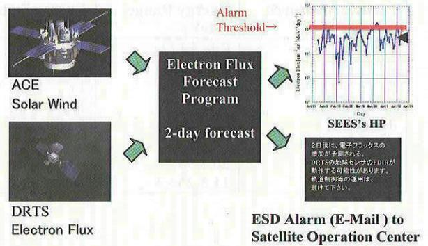
Fig. 6 High-Energy Electron Alarm System
