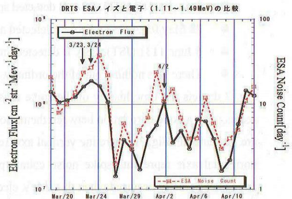
Fig. 2 Correlation between the DRTS /ESA spike noise (broken line) and the electron flux (1.1 to 1.5 MeV) (solid line) measured on board the same satellite. Anomalies on ESA are indicated by arrows.
