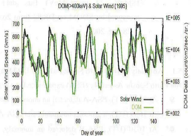
Fig. 4 ETS-V satellite DOM (dosemeter) electron flux (>400 keV) and solar wind speed (WIND: NSSDC) correlation[7].
