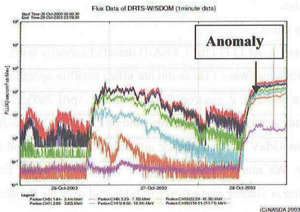
Fig. 1 Proton (1.4 to 2MeV, 3.7 to 5MeV, 8 to 18MeV, 22 to 45MeV) flux data measured by SDOM on DRTS from 26 to 28 Oct. 2003.
