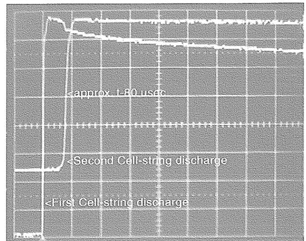
Figure 4: SSP-1 voltage traces, red and blue strings
