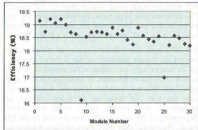
Figure 3: GaAs Module Efficiencies
