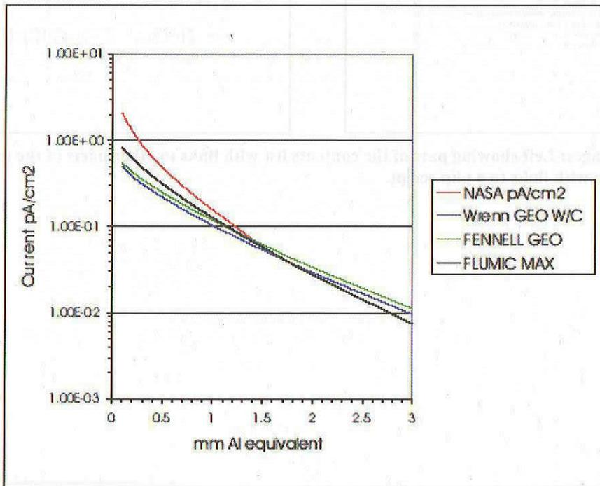
**Figure 4 Incident current as a function of shielding thickness for worst case spectra for geostationary orbit, comparing FLUMIC [2] for L=6.9, the NASA worst case spectrum [3], Wrenn et al's 'worst case' spectrum [2] and Fennell et al's [4] worst case environment. The FLUMIC spectrum was the maximum of the solar cycle, nominally 14th April 1994.**
