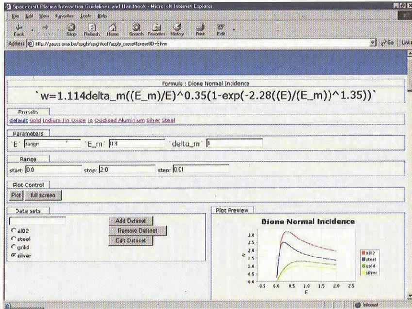
Figure 6 Example of calculation of a secondary electron yield using an equation by Dionne for normal incidence.
