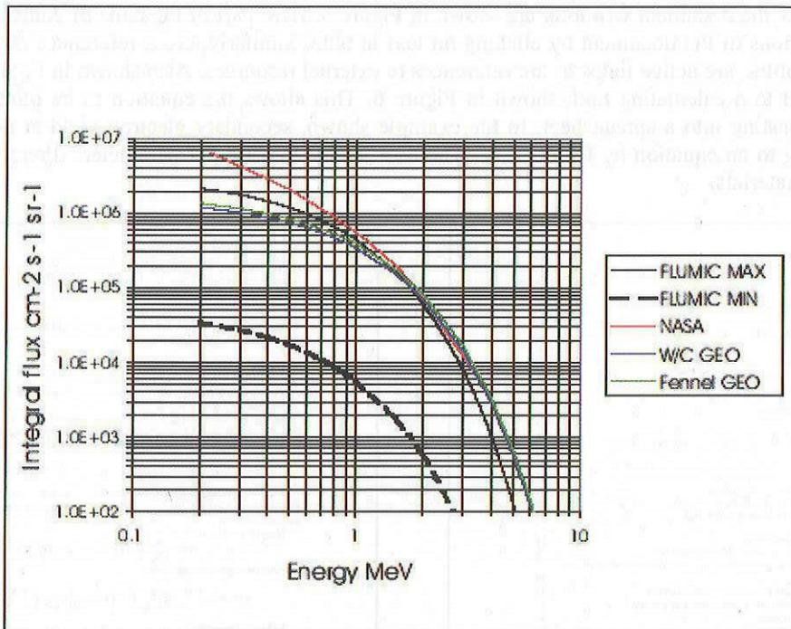
**Figure 3 Worst case spectra for geostationary orbit, comparing FLUMIC [2] for L=6.9, the NASA worst case spectrum [3], Wrenn et al's 'worst case' spectrum [3] and Fennell et al's [4] worst case environment. Approximate maximum and minimum values for FLUMIC correspond to 14th April 1994 and 21st December 1989 respectively.**
