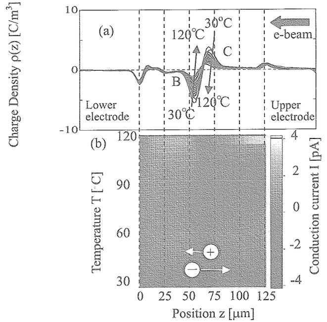
Fig.8 Temperature dependent (a) the charge and (b) the conduction current distributions in polyimide film irradiated by e-beam for 600s.
