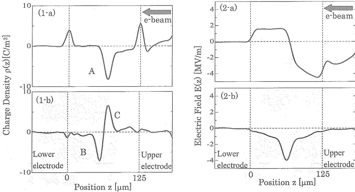
Fig. 4 Charge (1) and electric field (2) distributions in e-beam irradiated polyimide film for (a) 10, and (b) 600s, respectively.
