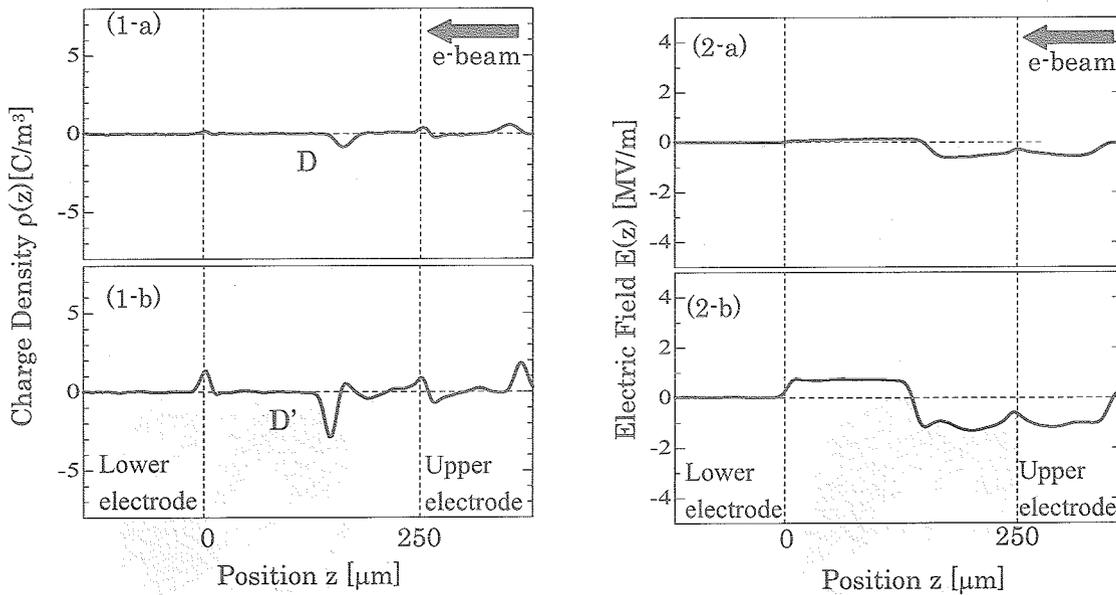
Fig.5 Charge (1) and electric field (2) distributions in e-beam irradiated polystyrene film for (a) 10, and (b) 600s, respectively.
