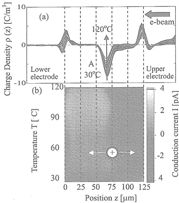
Fig.7 Temperature dependent (a) the charge and (b) the conduction current distributions in polyimide film irradiated by e-beam for 10s.
