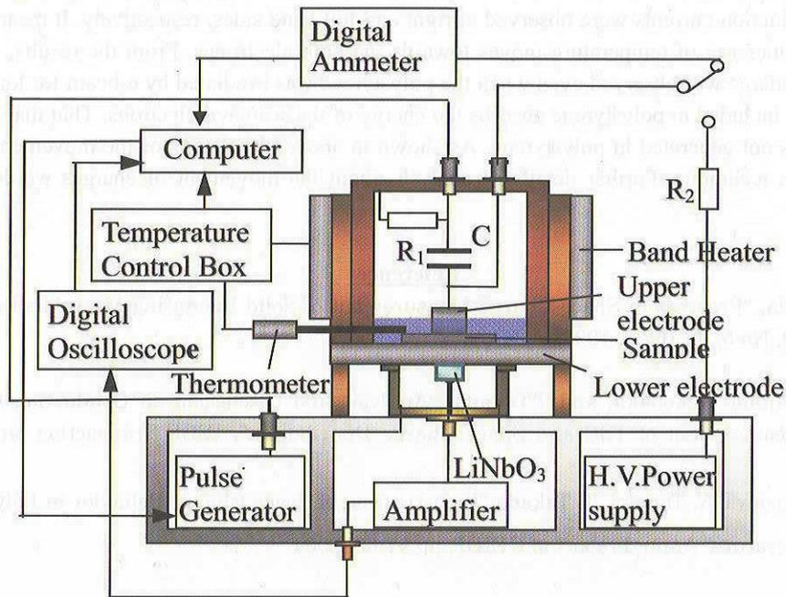
Fig.3 Measurement system for internal charge distribution during elevating temperature
