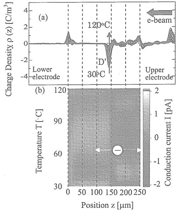
Fig.10 Temperature dependent (a) the charge and (b) the conduction current distributions in polystyrene film irradiated by e-beam for 600s.
