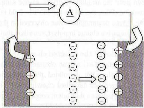
Fig.2 Principle of thermally stimulated current (TSC)
