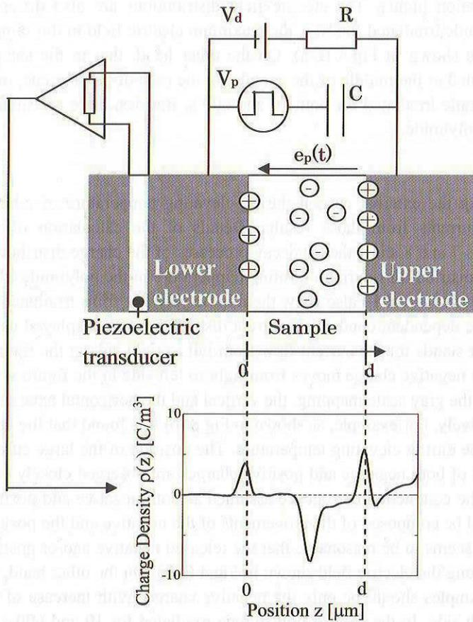
Fig.1 Principle of the PEA method
