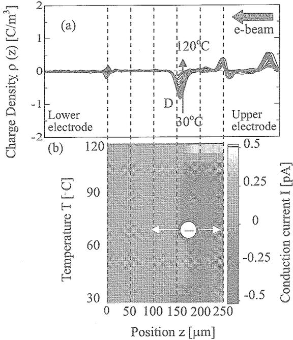
Fig.9 Temperature dependent (a) the charge and (b) the conduction current distributions in polystyrene film irradiated by e-beam for 10s.
