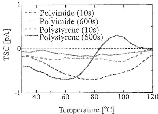
Fig 6. TSC curves obtained by measuring the external current during elevating temperature of e-beam irradiated samples.
