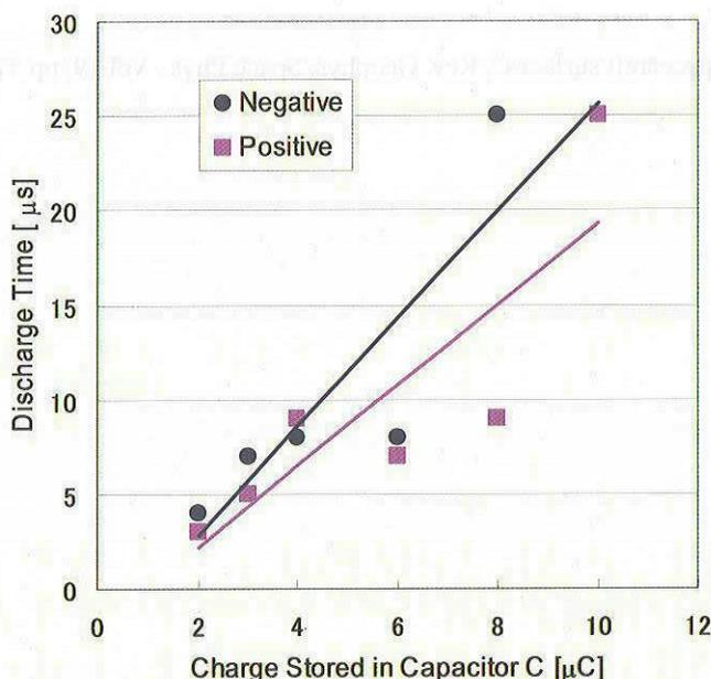
Fig.5 Dependence of discharge time on the charge quantity stored in capacitor.
