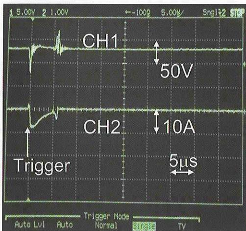
(a) Waveforms of voltage and current
