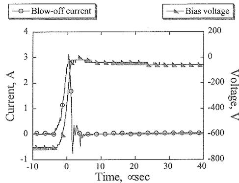
Figure 6. Typical waveform of the blow-off current and the bias voltage when a primary arc occurs
