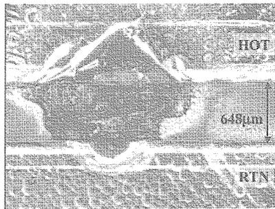
Figure 10. Destroyed gap by the permanent sustained arc
