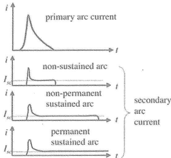
Figure 2. Definition of arc current
