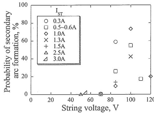
Figure 12. Change of non-permanent sustained arc occurrence according to the string voltage
