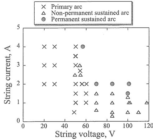
Figure 11. Mapping of the threshold voltage and current to induce secondary arc
