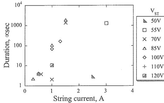
Figure 13. Change of non-permanent sustained arc duration according to the string current
