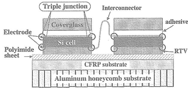
Figure 1. Solar array structure
