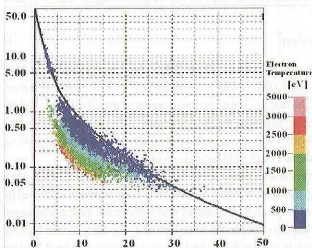
Figure 2. Characteristic of relationship between the spacecraft potential and the electron density in the near tail regions.
