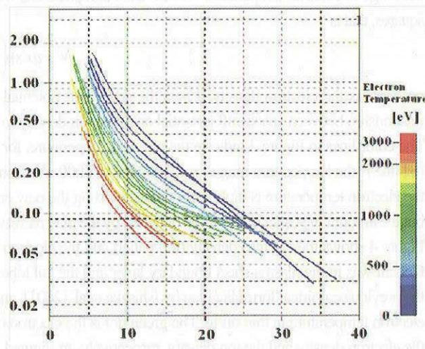
Figure 3. Approximate formula of relationship between the spacecraft potential and the electron density each electron temperature.
