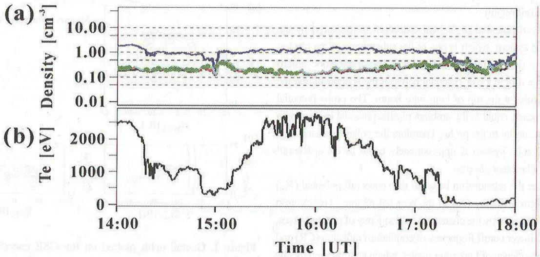
**Figure 4.** Electron density and electron temperature observed by the Geotail spacecraft at 14:00 – 18:00 UT, 30 January, 1997. (a) top panel : Electron density calculated by spacecraft potential with new empirical formula, measured by the LEP and estimated by the PWL, respectively. (b) bottom pane : Electron temperature measured by the LEP.
