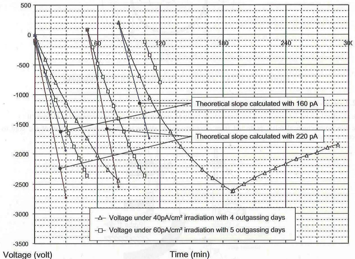
**Figure 8** Braid voltage of one peripheral coaxial line under 40 and 60 pA/cm<sup>2</sup> irradiation fluxes.
