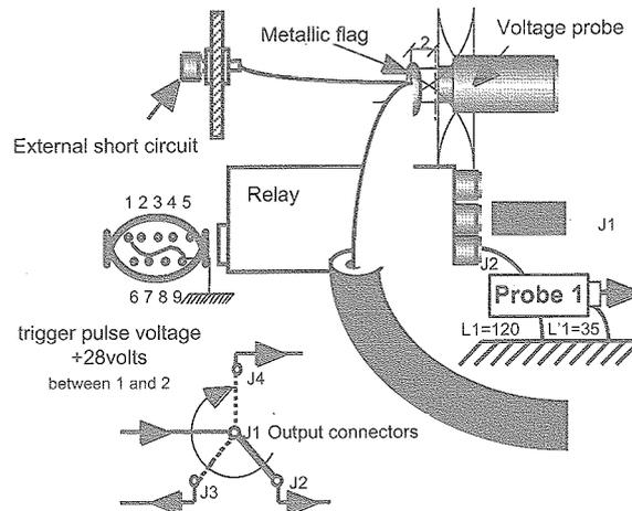
Figure 10 RADIALL® cable set-up with its associated instrumentation.
