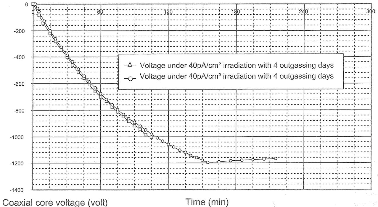
Figure 11 Core voltage variation versus time under a  $40 \text{ pA/cm}^2$  irradiation flux Radiall® coaxial cable.
