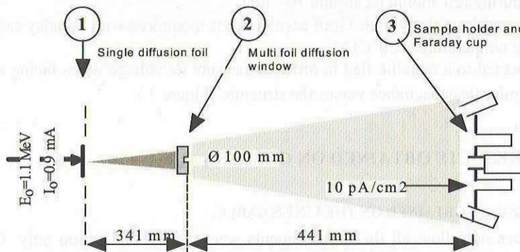
Figure 2 GEODUR Schematic set-up
