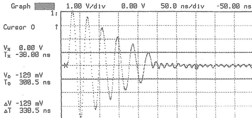
Figure 12 Current transient monitored on a Pearson probe during a discharged triggered when switching relay (charging potential: -1000V – probe transfer function  $1\text{V}=2\text{A}$ ).
