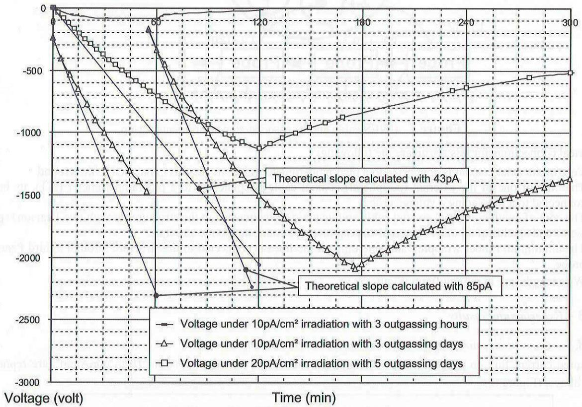
**Figure 7** Braid voltage of an external cable under electron irradiation (10 and 20 pA/cm<sup>2</sup>) versus time.
