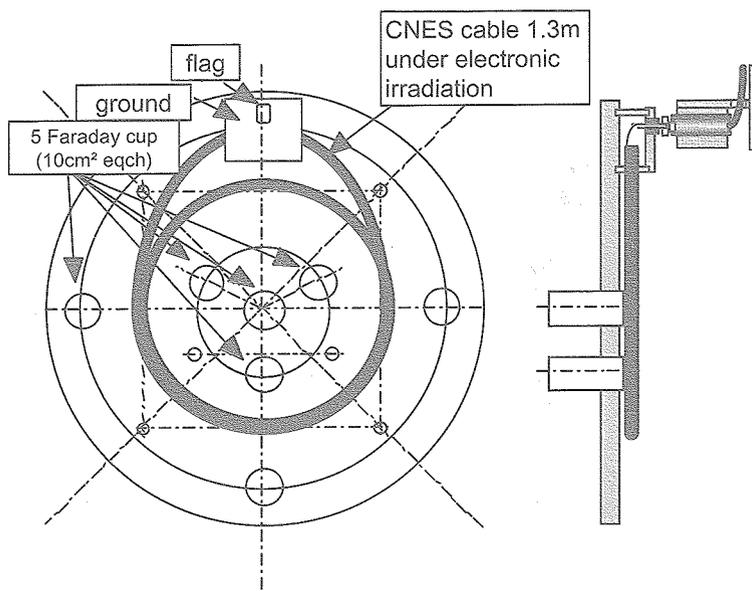
Figure 4 CNES cable assembly on the GEODUR samples-holder.
