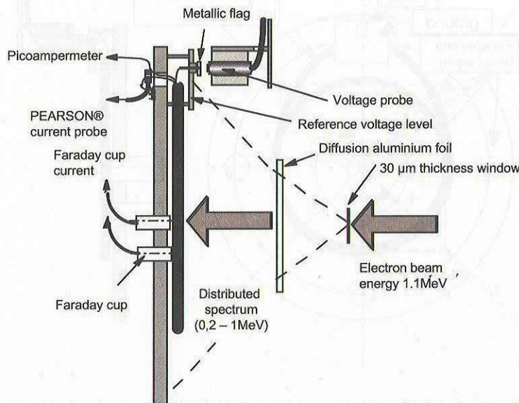
Figure 3 : Schematic view of the instrumentation around the GEODUR sample holder.
