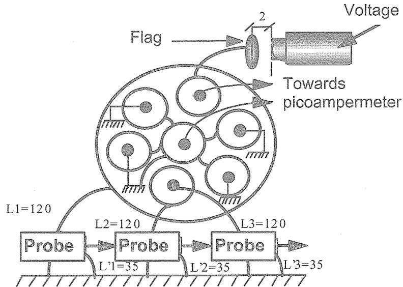
Figure 5 CNES cable and its associated measurements set-up.
