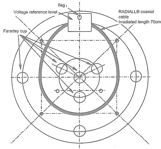
Figure 9 : RADIALL cable assembly on the GEODUR samples-holder
